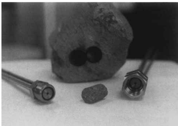
Figure 3. "G" Tunnel tuff, cored sample, and diffusion cell parts.
